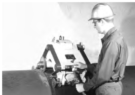
Cutting ductile iron pipe with milling cutter.
