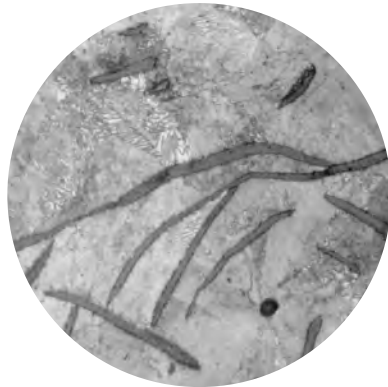
Photomicrograph showing graphite form in gray iron.
